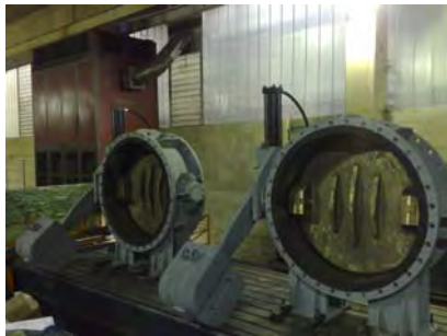
VALVES ND 52" USED FOR PUMP PROTECTION WITH BODY RUBBER COATED AND DISC IN BRONZE-ALUMINIUM
