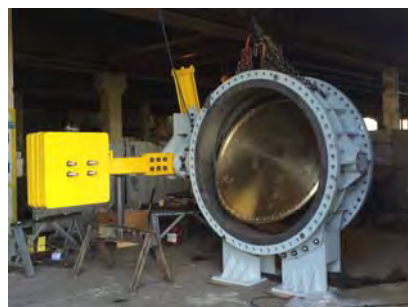
NO. 6 VALVE ND 72" USED FOR PUMP PROTECTION WITH BODY RUBBER COATED AND DISC IN BRONZE-ALUMINIUM
